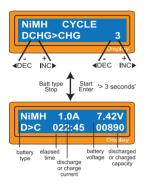
Set the sequence on the left and the number of cycle on the right. You can use this function for balancing, refreshing and break-in the battery. To avoid rising temperture of the battery, there will a brief cool-off period that already fixed at 'User setting' after each charge and discharge process. The cycling number ranges from 1 to 5.
