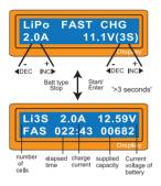
You can set up the charging current and the voltage of the battery pack being charged. As you press Start/ Enter button the voltage confirmation will be displayed. And then, if you confirm the voltage and current, press Start/ Enter button again to start charging.
