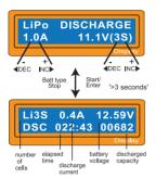
The value of discharge current on the left side of screen may not exceed 1C for a maximum safety and the final voltage on the right should not be under the voltage level that is recommended by the battery manufacturer to avoid deep discharging.
