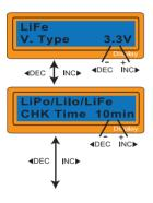
The screen displays the nominal voltage of Lithium battery. There are three kinds of Lithium battery; LiFe(3.3V),Lilo(3.6V) or LiPo(3.7V). This is very important so you have to check the battery carefully and set it up correctly. If it is different from correct value the battery can explode during charge process.
