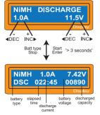
Set discharge current on the left and final voltage on the right. The discharge current ranges from 0.1 to 1.0A and the final voltage ranges from 0.1 to 25.0V). To start the process, press Start /Enter key more than 3 seconds
